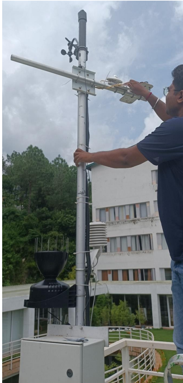
Figure 10: CEEST Automatic Weather Station installed at Shoolini University. The weather station is equipped to monitor solar radiation, temperature, humidity, photosynthetic active radiation as well as wind speed and direction.
